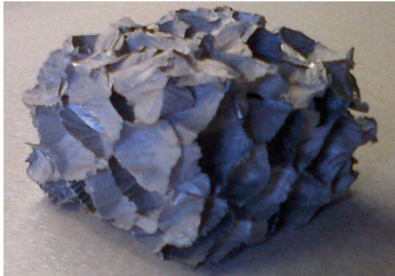
Fig. 13.2 Aluminium foam with a narrow Gaussian-like distribution of void sizes of around 1 cm diameter partially wrapped in fragmented metallic shells, used as crushable buffers inside vehicle bodies. The cosmological void distribution is by contrast gamma-like with a long tail [8], interspersed with 60% of galaxies in large-scale sheets, 20% in rich filaments and 20% in sparse filaments [12]. Such 3D stochastic porous materials can both be studied by tomographic methods, albeit at different scales by different technologies, yielding sequences of 2D stochastic texture images
