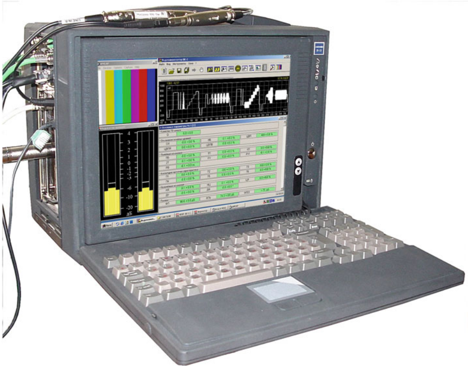
Fig. 2. Systems for TV measurements KI-TVM, KI-TVM- E (reference) and KI-TVC
