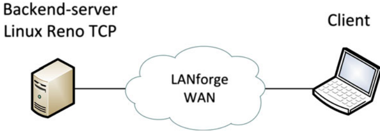
Fig. 1. The logical diagram of the network topology used for TCP throughput measurements.
