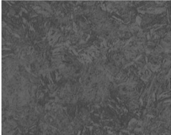
Fig. 6 Microstructure of high strength steel bolt material after tempering process
