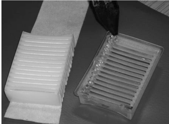
Fig. 2 Assembly of filter glued with hot glue
