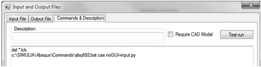
Fig. 7 Command line for execute of Abaqus
