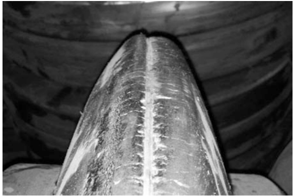
Fig. 3 Wear of straightener straightening rolls
