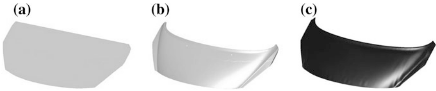
Fig. 2 Process of transforming cloud of points into surface using example of a car's bonnet
