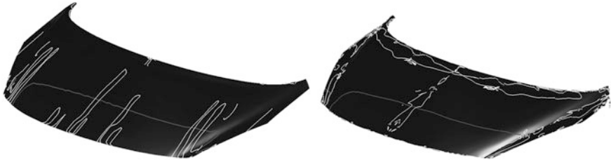
Fig. 3 Two models of a car’s bonnet, made by using different algorithm, with analysis of reflection (grey colour) and inflection lines (white colour)
