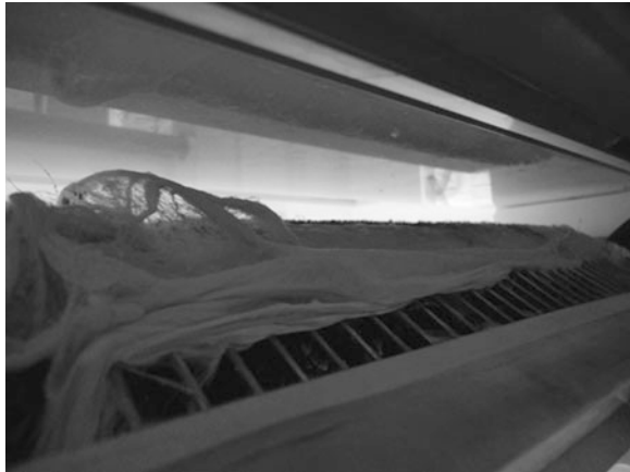
Fig. 5 Pulled down layer of fibers
