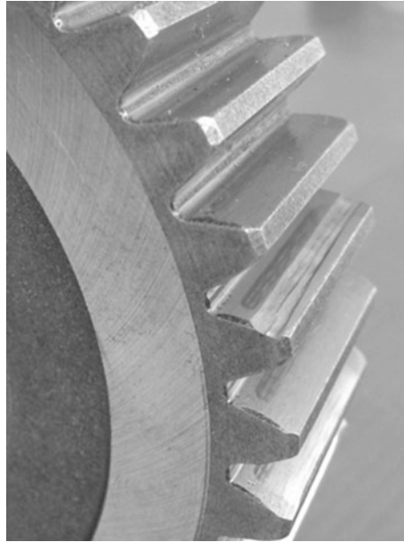
Fig. 3 Damaged sprocket of the first planetary row central wheel on the transmission A2000
