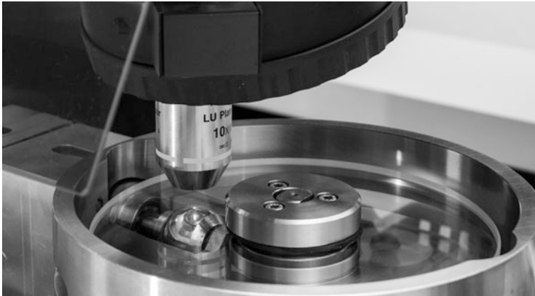
Fig. 3 Detail of the contact between steel ball and glass disk
