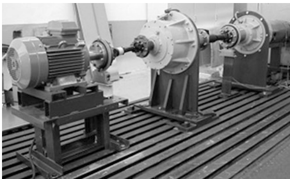
Fig. 1 Testing unit KKaČS for gears tests
