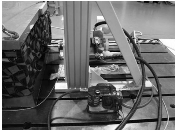
Fig. 3 Hydraulic cylinder AH 25-250
