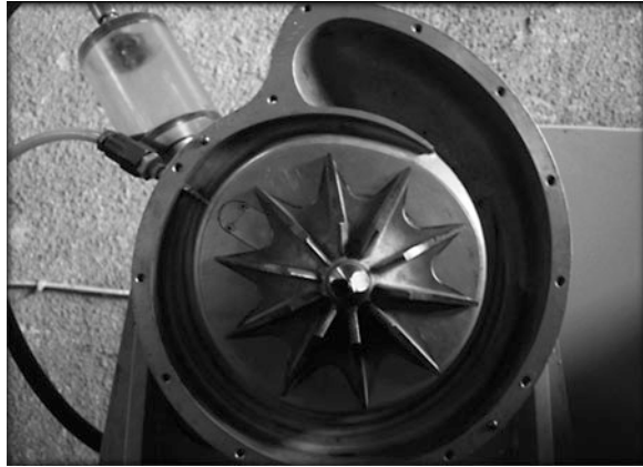
Fig. 3 Impeller and volute of centrifugal compressor
