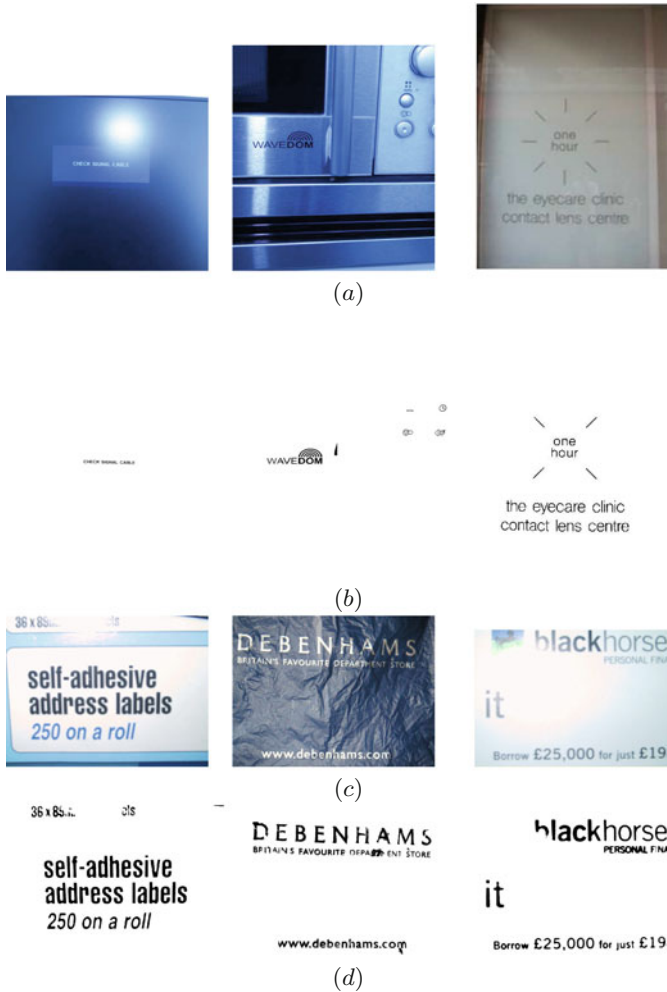
Fig. 12. (a) & (c) A few samples from ICDAR 2003 robust reading competition database affected by non-uniform lighting or shadow, (b) & (d) results of the proposed method on respective image samples shown in (a) & (c).
