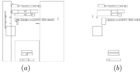
Fig. 4. (a) Bounding rectangles of connected edge components obtained from the image of Fig. 1(a), (b) candidate text regions of the sample of Fig. 1(a).
