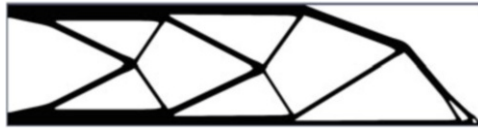
Fig. 6 A long cantilever beam with low material fraction and a low interfacial energy penalization
