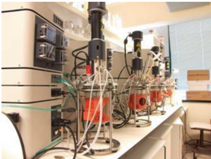
Fig. C.1 Expansion of human mesenchymal stem cells in stirred-tank bioreactors (Courtesy of Stem Cell Bioengineering Laboratory, IST)
