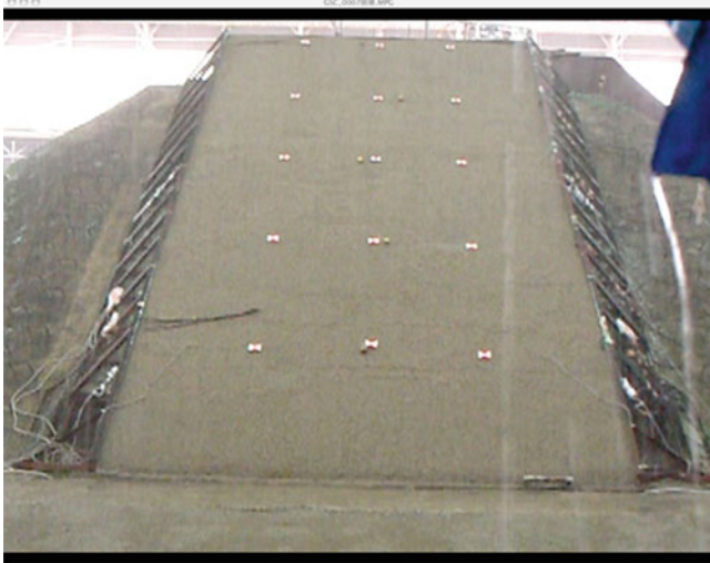
Fig. 7 Picture of model slope about 1 min before failure in experiment No. 4
