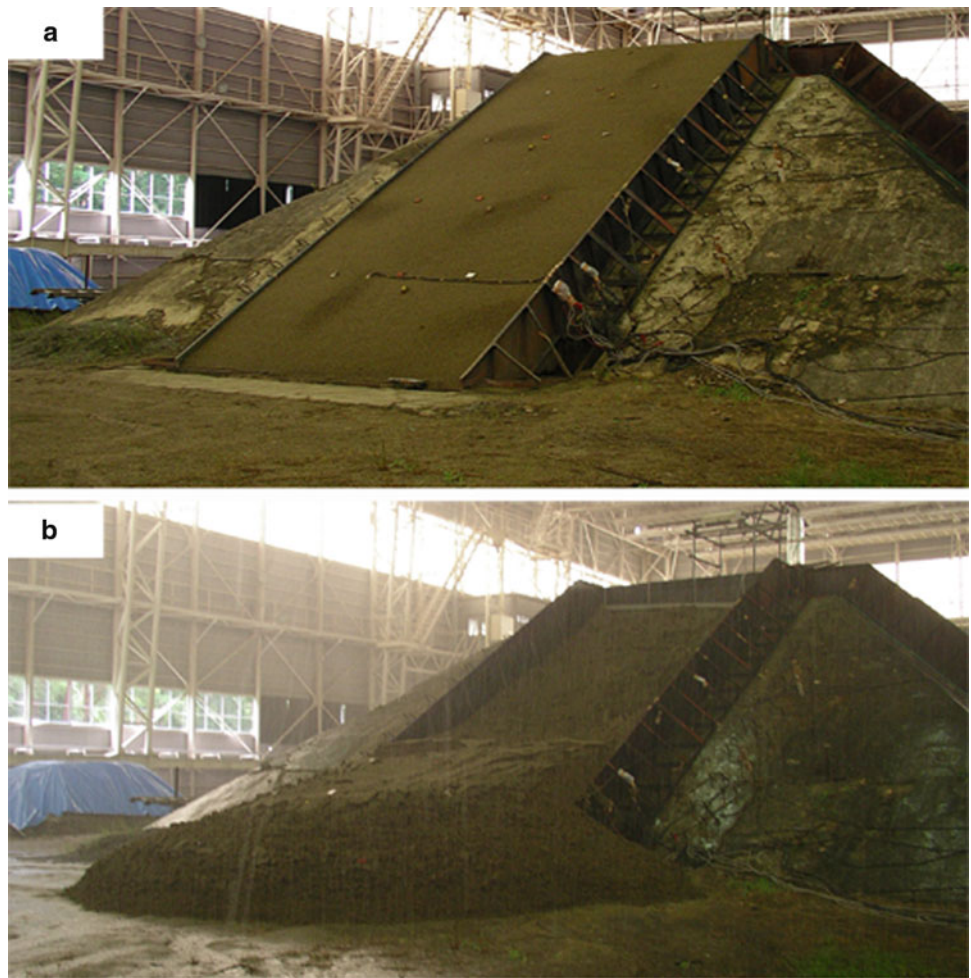
Fig. 3 Model slope used in experiments No. 1–7. (a) Before failure; (b) after failure
