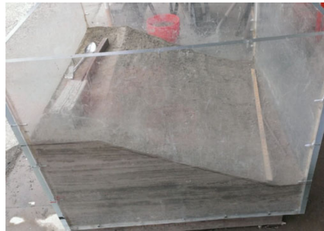
Fig. 15 Photograph of the slope model after its completion
