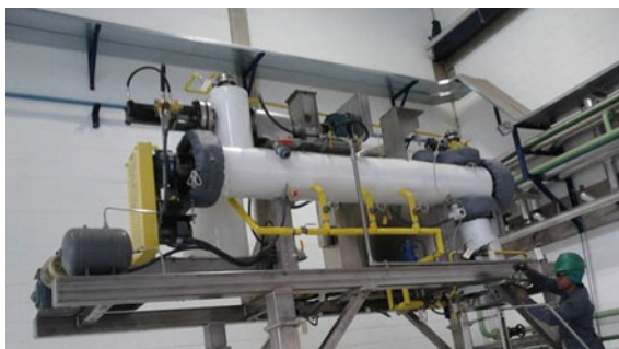
Fig. 11.5 Continuous reactor of steam explosion AdvanceBio LLC-USA with a capacity of 75 kg.h -1
