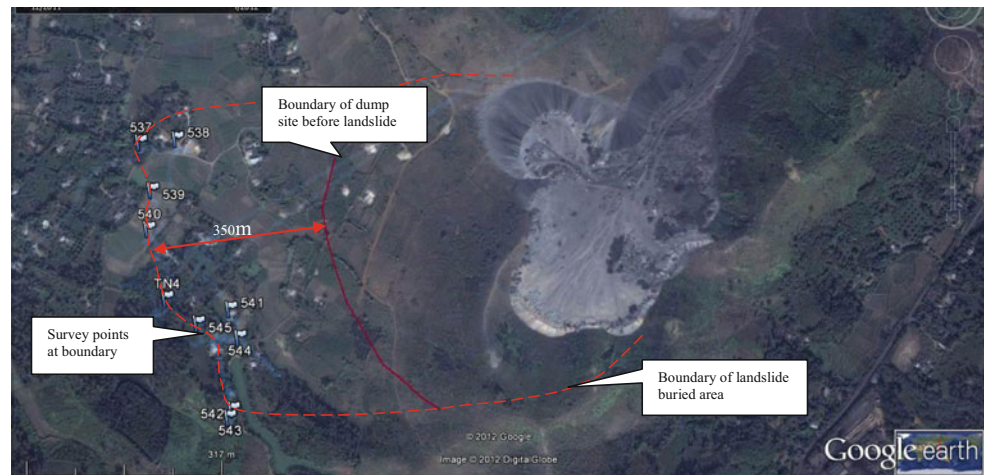
Fig. 4 Boundary of the landslide before and after event
