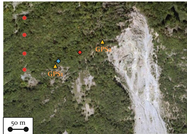
Fig. 1 Top view of the site (©Google): seismic sensors in the gallery (red dots), GPS stations (triangles), and boreholes for hydrological (blue diamond) and microseismic (red diamond) measurements
