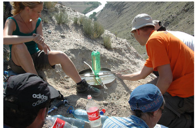
Fig. 4 Participants of the 2011 Summer School performing an in-situ permeability test at the comminuted lower part of the Kokomerren rockslide deposits. Plastic bottles were used to bring sufficient water to the site, which is about 150 m above the river
