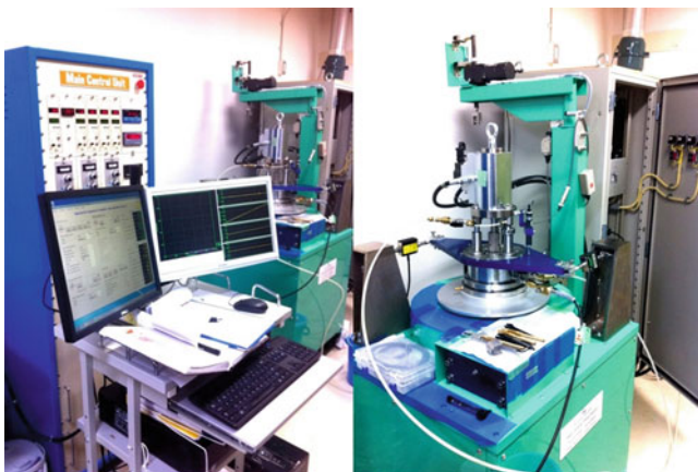
Fig. 3 The overview of the undrained dynamic loading ring shear apparatus ICL2
