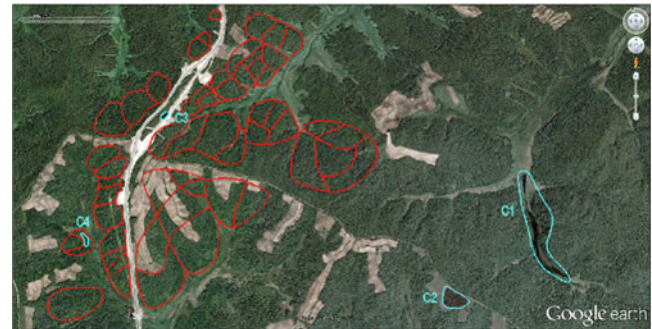
Fig. 4 Creeping surfaces and the distribution of melting permafrost in study area
