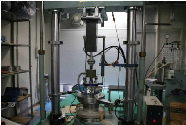
Fig. 4 The ring shear apparatus
