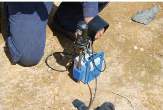
Fig. 5 Using a penetrometer to determine the depth of the possible failure
