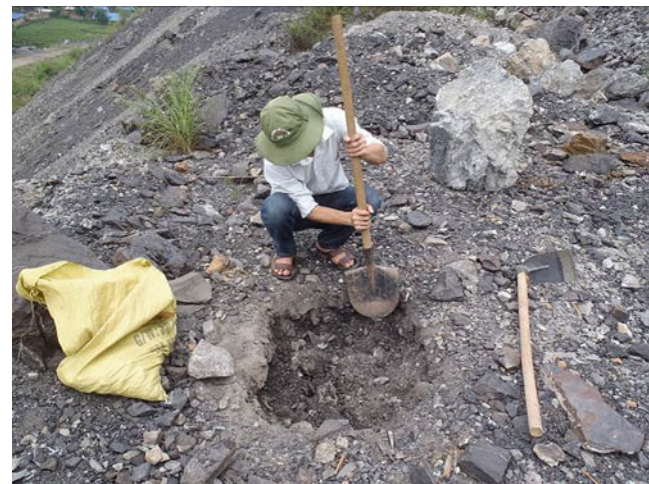
Fig. 2 Determine in-situ density of waste materials by digging hole
