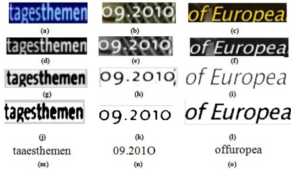
Fig. 4 (a),(b),(c) Sample CCs (d),(e),(f) Median Filter output (g),(h),(i) Background eliminated CCs (j),(k),(l) Binarized output (m),(n),(o) OCR output
