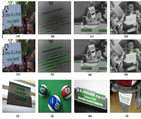
Fig. 5 (a),(b),(c),(d) Text Detection result for Yang method (e),(f),(g),(h) Text Detection result for proposed method (i),(j)Text Detection result for MSRA Database (k),(l) Text Detection result for own Database
