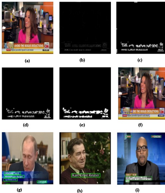
Fig. 2 (a) Original Video frame (b) Wavelet based Edge Map (c) Fuzzy C-means threshold output (d) SWT verification output (e) Morphological Operation output (f) Detected Text Region (g),(h),(i) Examples of text detection
