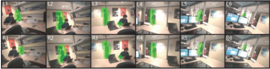
Fig. 6.18 A sequence of images recorded during the real time stereo tracking of a person walking in front of the iCub: six images are shown in temporal order from L1 to L6 ( left camera ) and R1 to R6 ( right camera ). The walking person is highlighted with a green blob using the result of proposed algorithm
