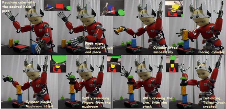
Fig. 7.9 Snapshots of the process of building the tallest stack from an available set of objects by combining past memories without any trial and error exploration
