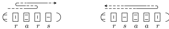
Fig. 1. Two systems composed of amplifiers ( a ), silencers ( s ) and reflecting silencers ( r ). On the left, the signal passes to the receiver provided that k \geq 3 , on the right, it returns back to the transmitter. The signal is normal in the dashed parts of the trajectory and amplified in the solid parts.
