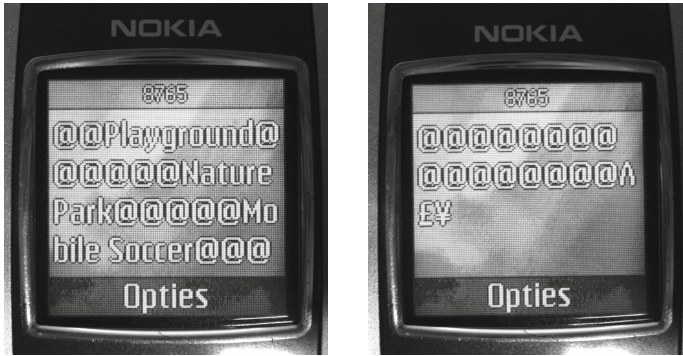
Fig. 5. These two pictures show the strange behavior when the same SMS is opened twice in a row. Note that the words in the left image are the names of games available on the device.
