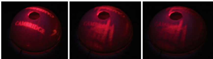
Fig. 1.24 Experimental images from the LC/antenna device. Left , 0 V applied ( vertical ). Centre , 0.44 \text{ Vum}^{-1} applied ( 45^\circ ). Right , 0.65 \text{ Vum}^{-1} applied ( horizontal )
