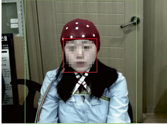
Fig. 2 Face detection results using Adaboost. ( Red Detected facial region, Green Defined candidate region of bust micro-movement)
