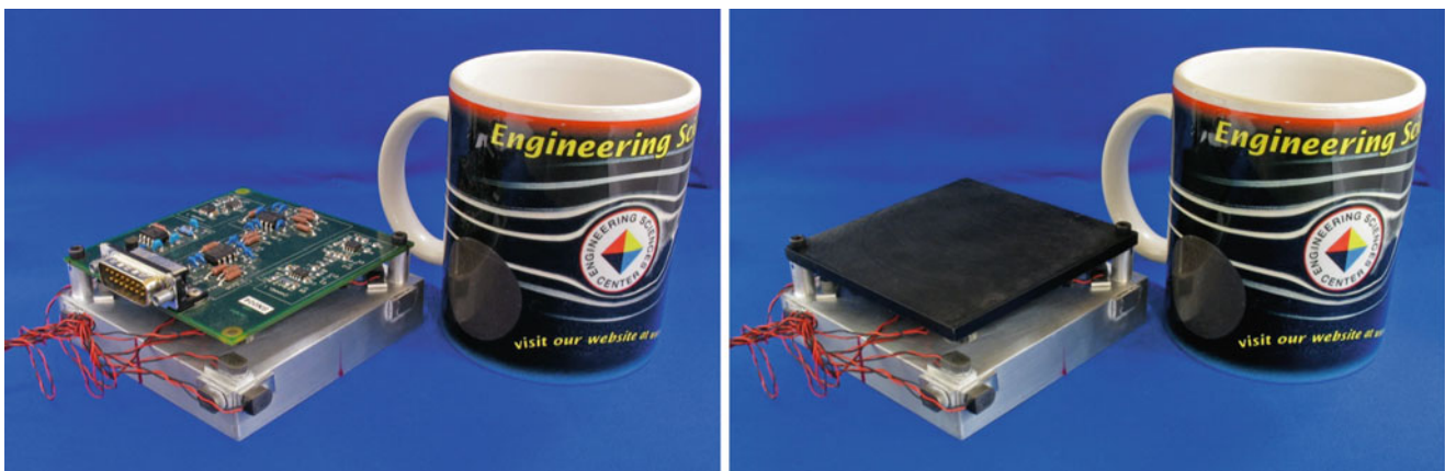
Fig. 21.1 Circuit board and fixture (left), truth plate and fixture (right)
