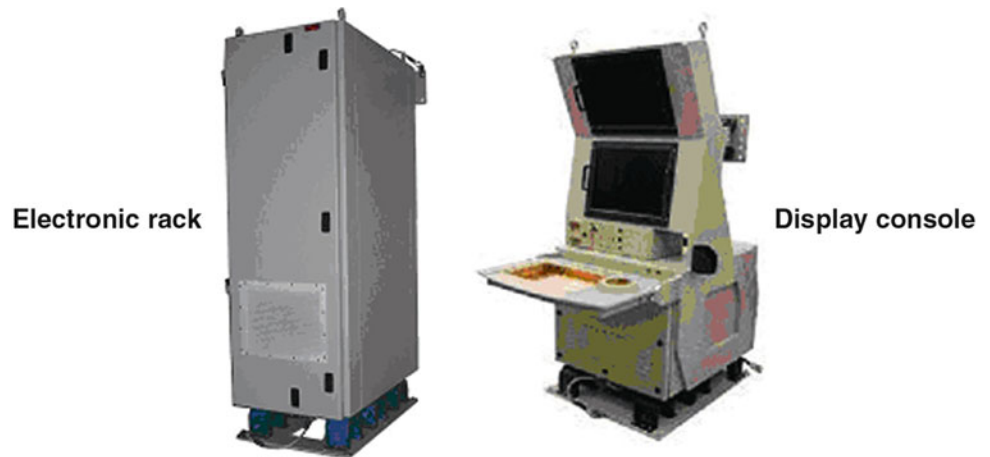
Fig. 11.1 901D LLC isolated rack and display console
