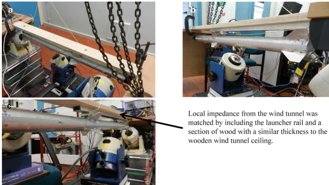
Fig. 37.12 Impedance Matched Multi-Axis Test for dummy missile. (a) IMMAT—view from above test setup. (b) IMMAT—view from tail of the missile. (c) IMMAT—view from below test setup
