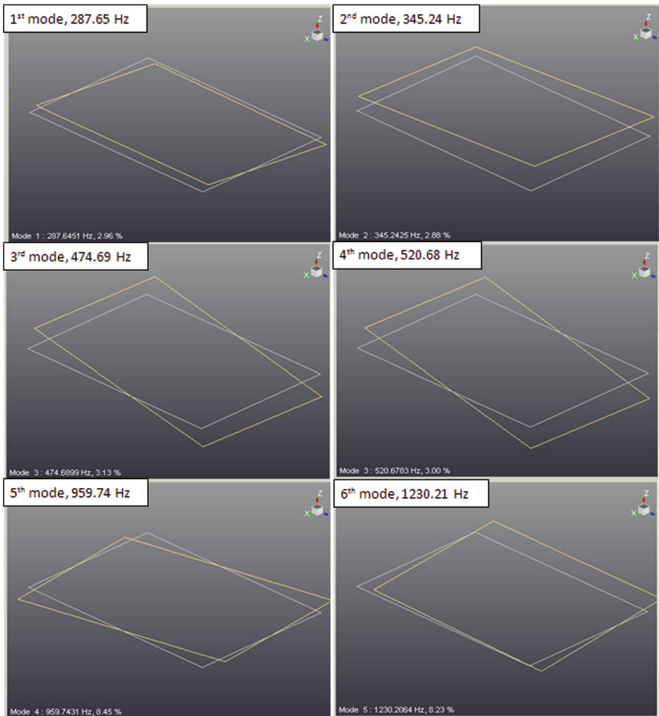
Fig. 32.9 First six natural frequencies and corresponding mode shapes of gyroscope B from modal tests, washers used
