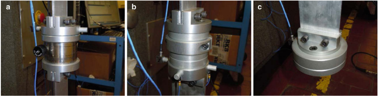
Fig. 34.3 Details of the test-rig: (a) first added mass with rotating graduated device; (b) second added mass with fixing device; (c) third added mass
