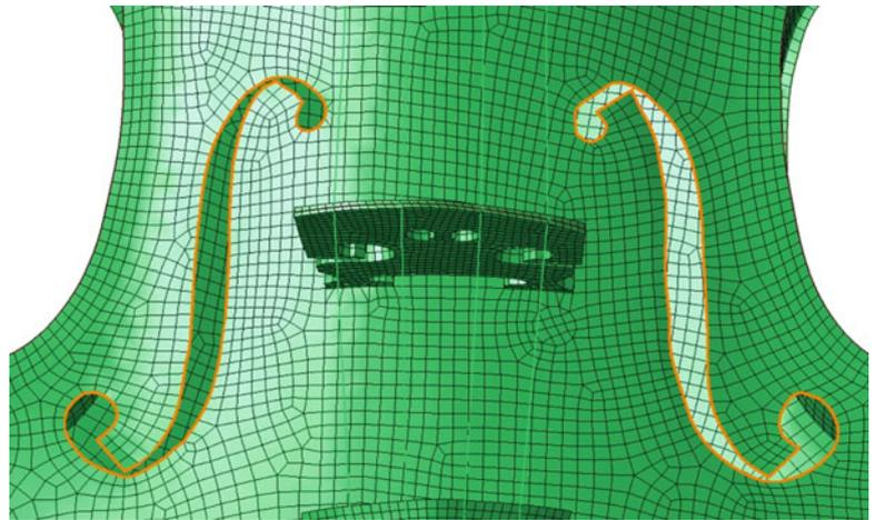
**Fig. 33.7** Final volumize mesh of the *Titian* Stradivari violin and cut-plane at bridge location
