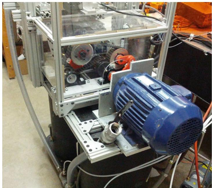
**Fig. 11.1** Engine test stand assembly
