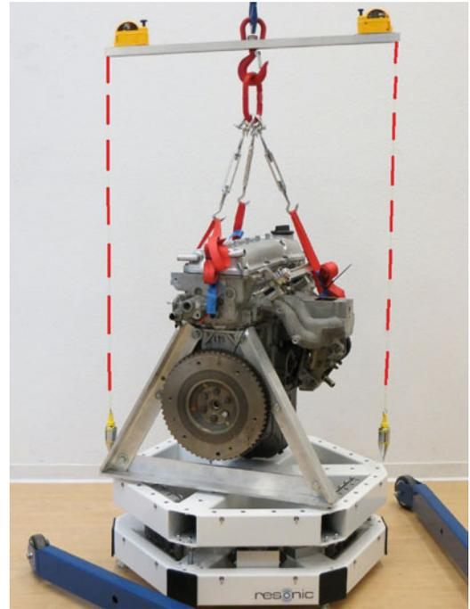
position, the test object's COG is at the platform center. (Both the plumb lines and the imaginary line connecting the hook and the COG are always vertical; therefore, given that the hook is at the center between the upper ends of the plumb lines, the  $x$  and  $y$  position of the COG is always at the center between the lower ends of the plumb lines.)
