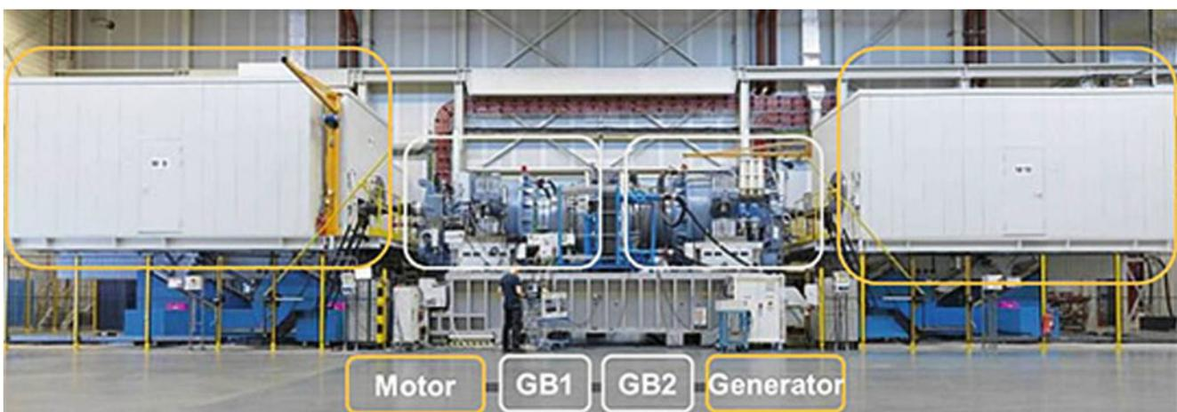
Fig. 5.1 ZF wind power test rig
