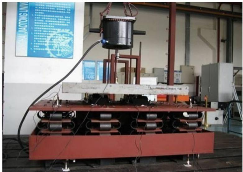
**Fig. 27.7** Measurement of the traditional absorber system
