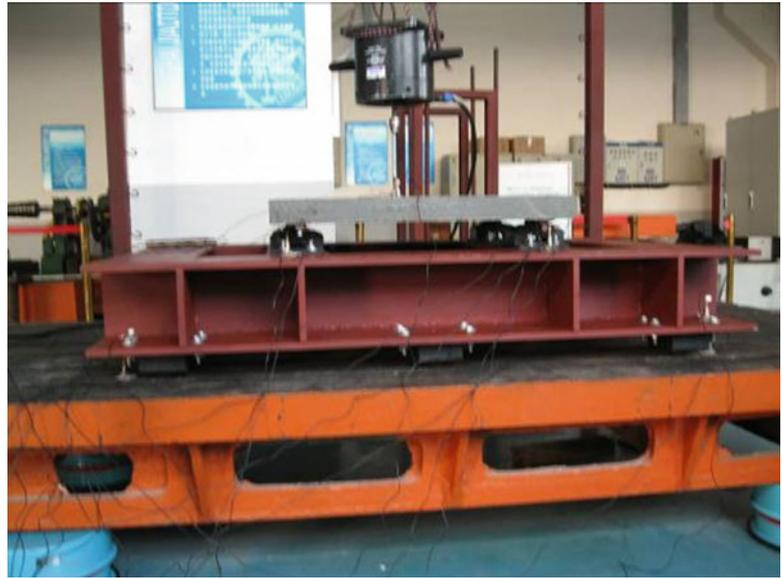
**Fig. 27.8** Placement of acceleration transducers on the absorber system
