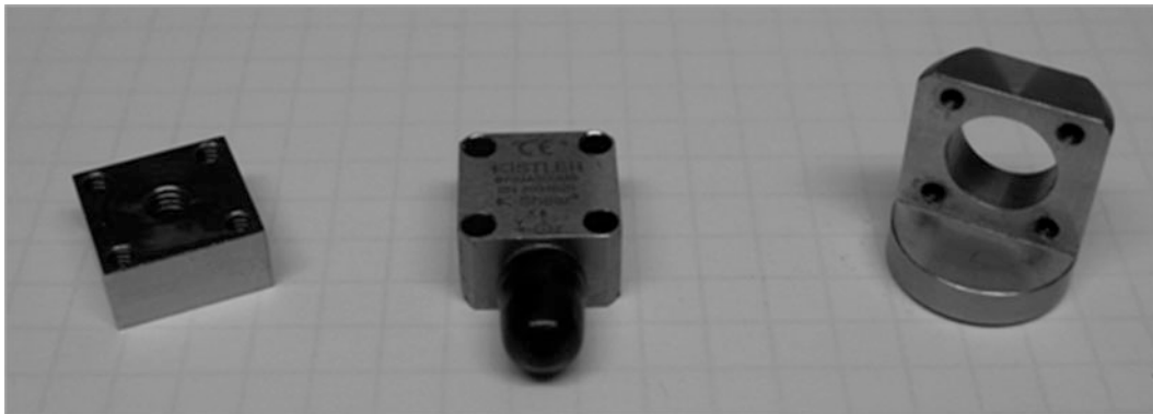
Fig. 28.2 Mounting adapters used to calibrate the z-axis ( left ) and the x- and y-axes ( right ) of a triaxial accelerometer Kistler type 8793A500 ( center )
