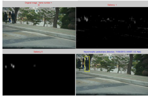
Fig. 19. Example image of successful pedestrian detection within a typical urban environment (consecutive image of Figure 18)
