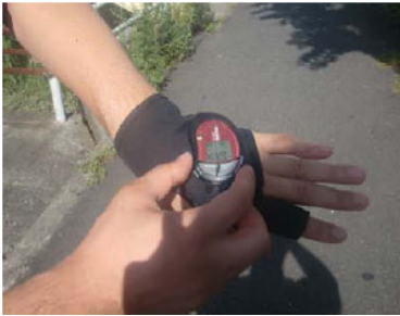
Fig. 4. Pulse rate sensor and examples of measured data
