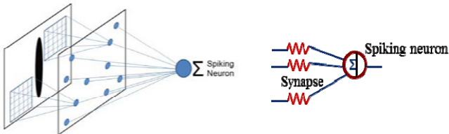
Fig. 3. Spiking neuron and neural networks to mimic the visual cortex's primary neuron
