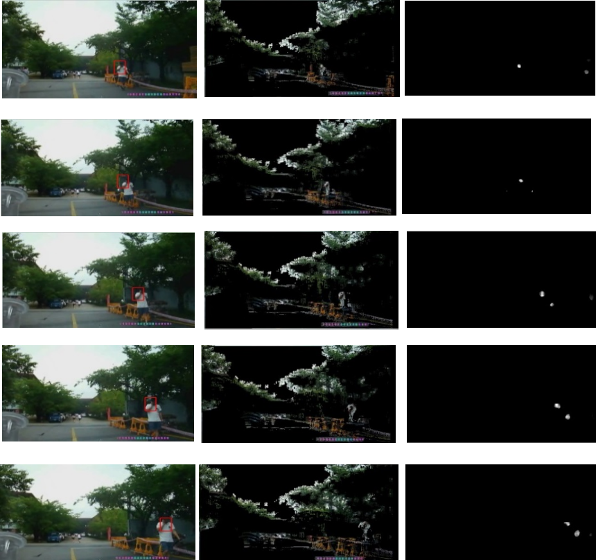
Fig. 29. Stereo neuromorphic processing of consecutive video frames at the rate of 30 frames/sec.(top to bottom) continuous frames until passing by the pedestrian,(left to right) input image with the detected location of head of pedestrian, disparity map, saliency map
