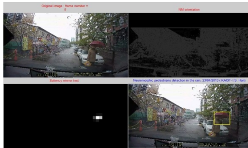
Fig. 17. Successful detection of a pedestrian with a hat and an umbrella, appeared from the street cars in the rainy weather.
