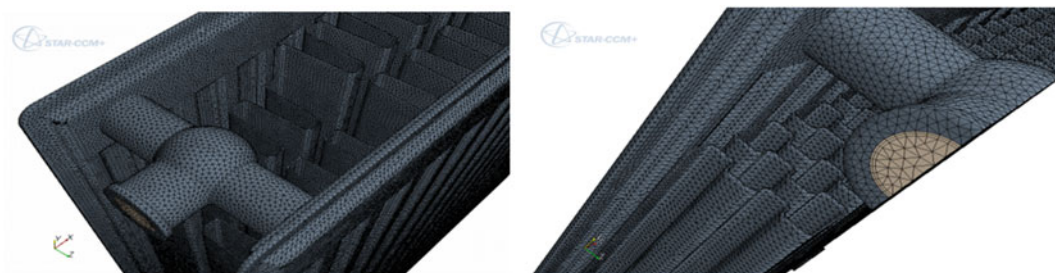
Fig. 58.4 Computational meshes of the panel radiator with original fin and new design-1
