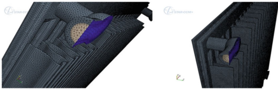
Fig. 58.5 Computational meshes of the panel radiator with new design-2 and triangular fin
