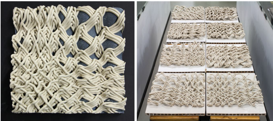
Fig. 6 Robotically printed panels prior to firing
