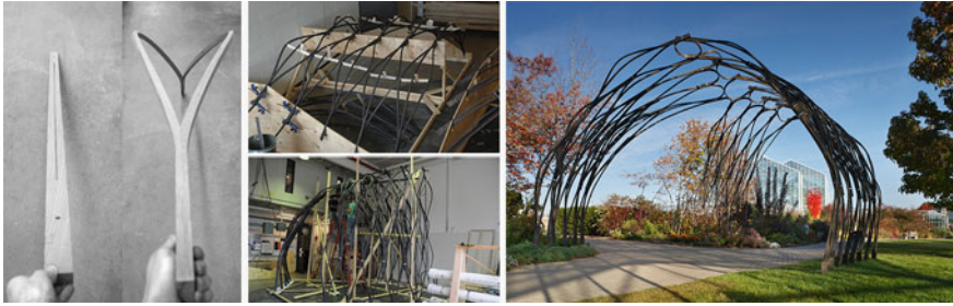
Fig. 1 Left water jet cut blank with registration holes, center materially intensive formwork for component assembly, right spring back installed
