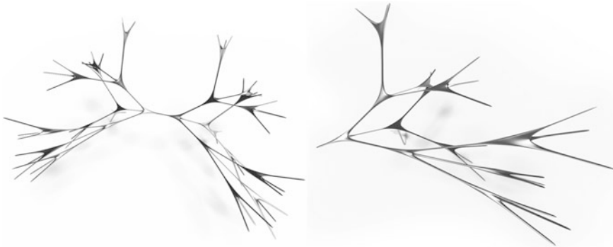
Fig. 10 Tree structures developed from parametric branching node definition
