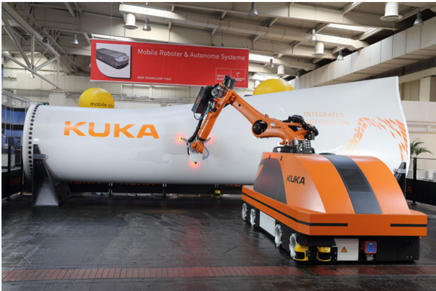
Fig. 4 KUKA moiros—mobile industrial robot system concept
