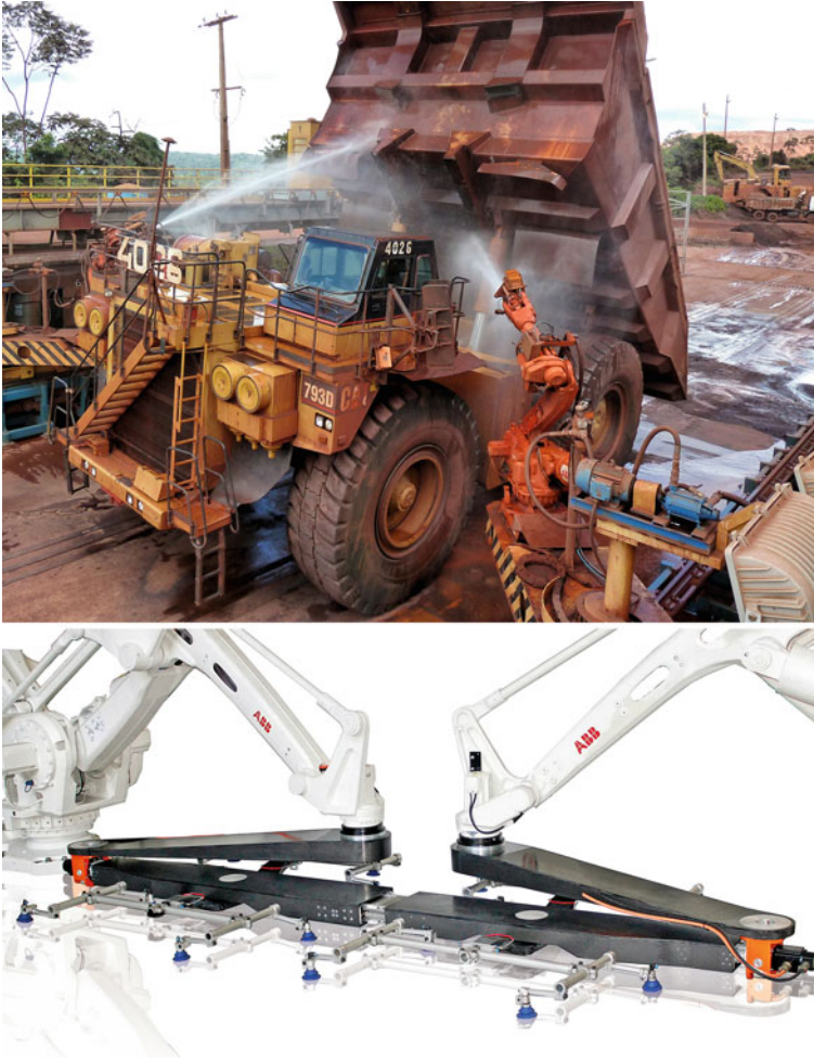
Fig. 2 Robotic truck washing ( above ), ABB TRX with cooperating robots for loading and unloading of large elements ( below )
