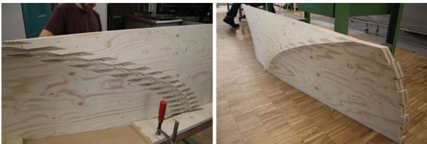
Fig. 8 Planar finger-type joints were used for the connections CV_1 – CX and CV_2 – CX . These joints were fabricated with a saw blade-slicing technique on a 5-axis CNC router
