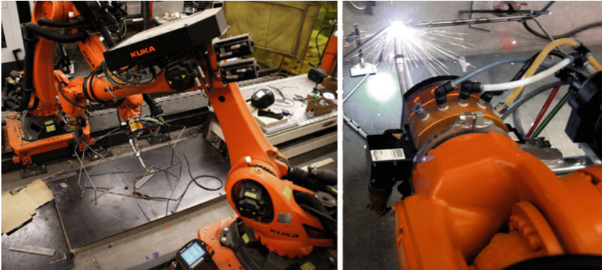
Fig. 3 Left Two Kuka KR120HA 6-Axis industrial robots with free-standing bender and shear, laser range-finder and MIG welding torch form a collaborative workcell for testing Adaptive Part Variation on steel rod assemblies. Right Welding in process
