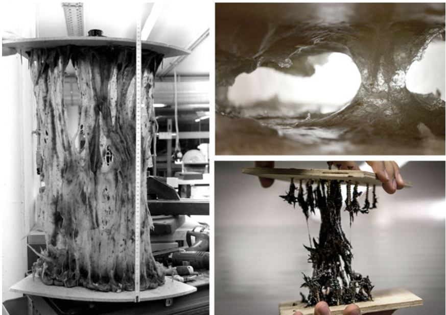
Fig. 3 “Thermoplastic stretching” material study utilizing polypropylene conducted during the course ‘Meeting Nature Halfway’. Images REXILAB
