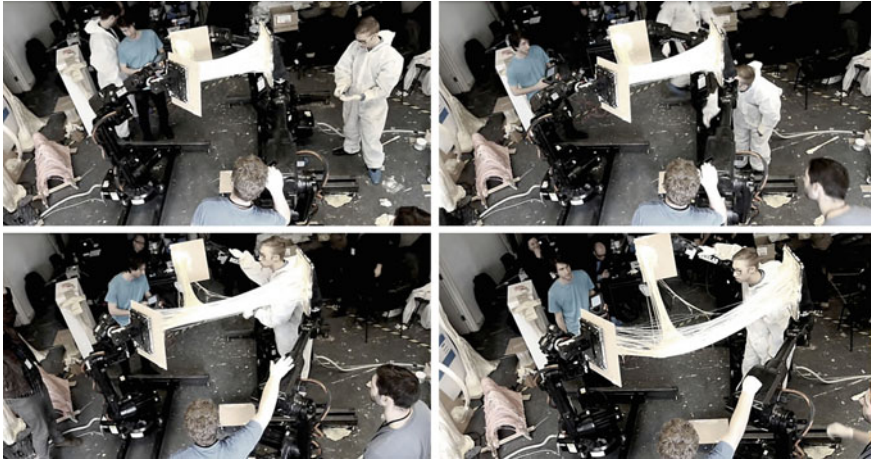
Fig. 1 Robotic foaming process exploiting for maximum dimension, conducted at Smart Geometry 2013. Images REXILAB
