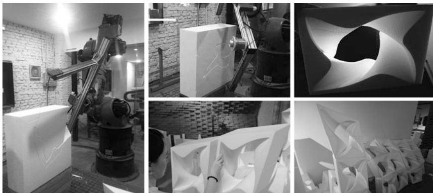
Fig. 5 Robotic fabrication and assembly process
