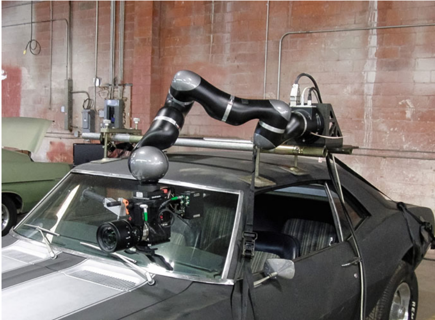
Fig. 2 CMOCOS using a KUKA lightweight robot as a car-mounted camera dolly for the Dreamworks movie Need for Speed
