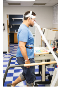
Fig. 2. The K-Sense evaluation environment where a person is walking on a treadmill in a metabolic lab
