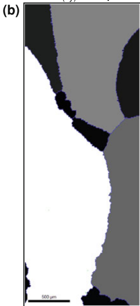
Fig. 15.6 a EBSD microstructure map for FeAl 28 , b microstructure map of misorientation angles between subgrains/grains
