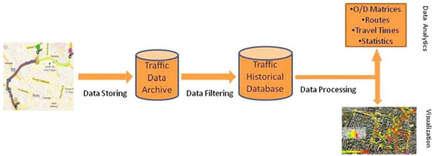
Fig. 1 Data acquisition, filtering and visualization workflow
