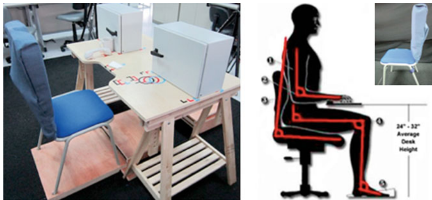
Fig. 141.1 The ADL Table Measurement left and the chair right designed to make the subject sit upright
