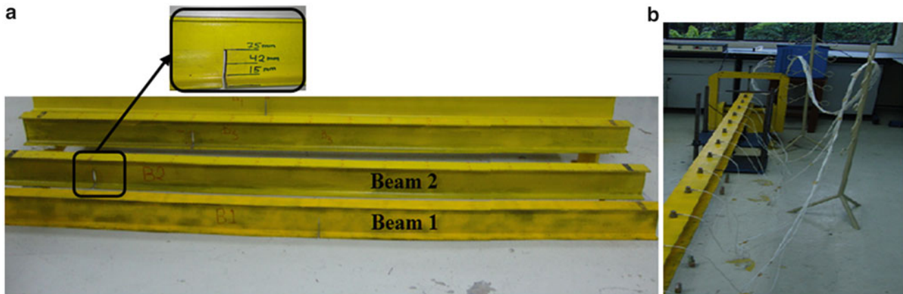
Fig. 25.4 Dynamic test in laboratory: (a) beams tested; (b) data acquisition
