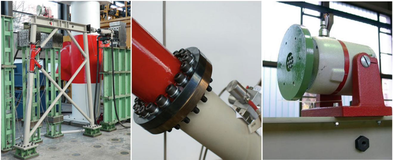
Fig. 19.3 Test stand for proof testing of damage identification algorithms; left : laboratory structure, middle : flange connection for damage modeling, right : electrodynamic shaker for excitation
