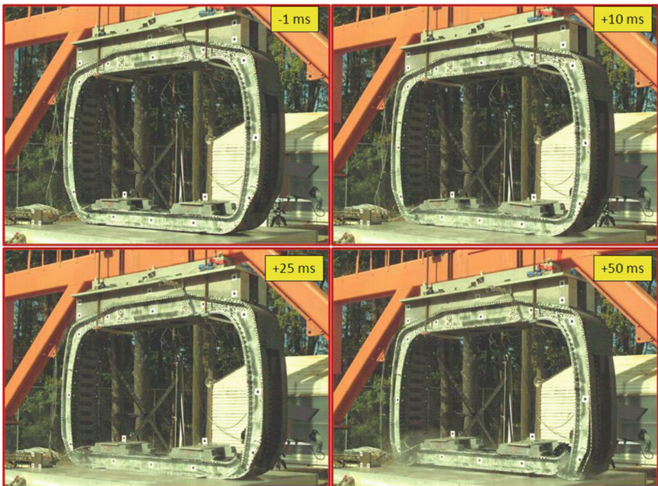
Fig. 7.8 Image sequence of the fuselage section drop test from the southeast camera
