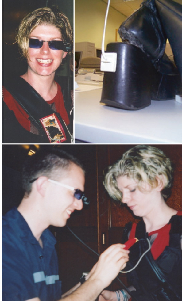
Fig. 16.1 My wearable computer with a MicroOptical head-mounted display (HMD) ( top left ) used at Art-Cels; platform boots with battery power ( top right ); and interacting with witting participants ( bottom ) (©2002 ..thePooch:.)
