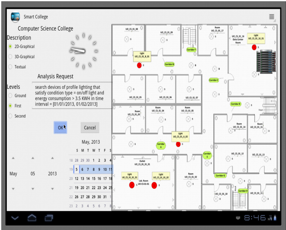
Fig. 4. Mobile Tool Interface for Energy Management in a Smart ICT Building
