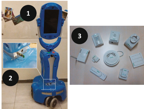
Fig. 9. The robot and the sensors used: 1) The GiraffPlus robot, 2) The ZigBee dongle connected to the robot, and 3) The environmental sensors
