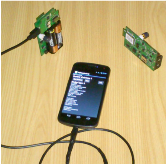
Fig. 2.13 Picture of the extended wireless sensor network setup
