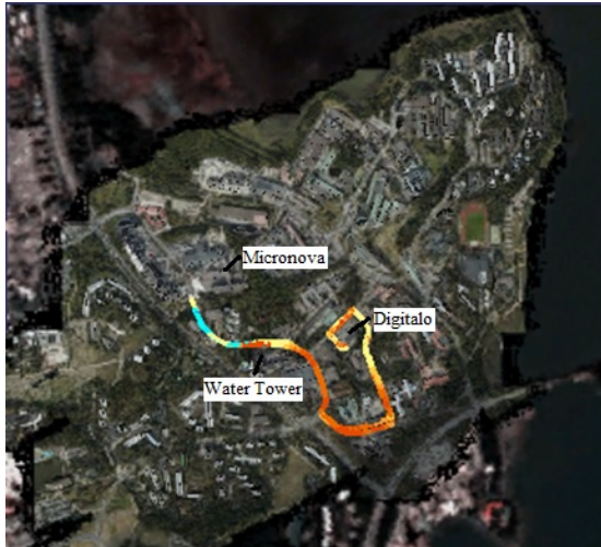
Fig. 7. Measurement route with signal strength colours
