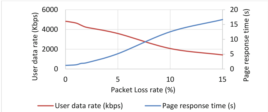
Fig. 10. Effect of the packet loss rate on the user data rate and the web page response time
