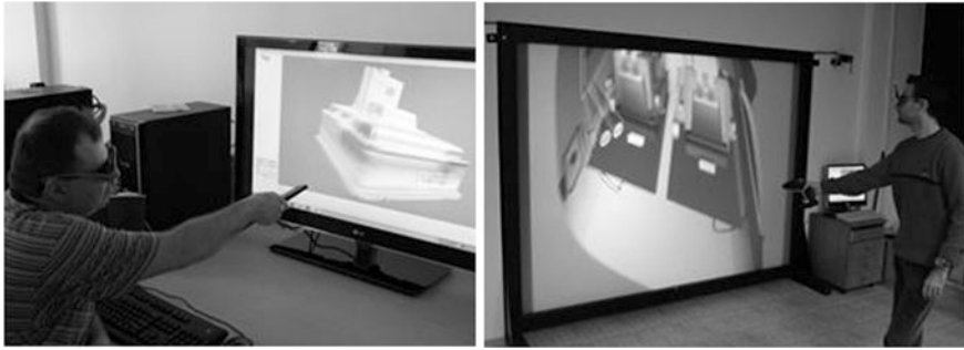
Fig. 6 Hardware configurations for implementation of implicit features exploration in VR environment: single desktop system (left) and cluster system with powerwall (right)
