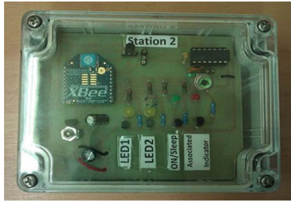
Fig. 2 Hot water system monitoring—light intensity and temperature monitoring [19]
