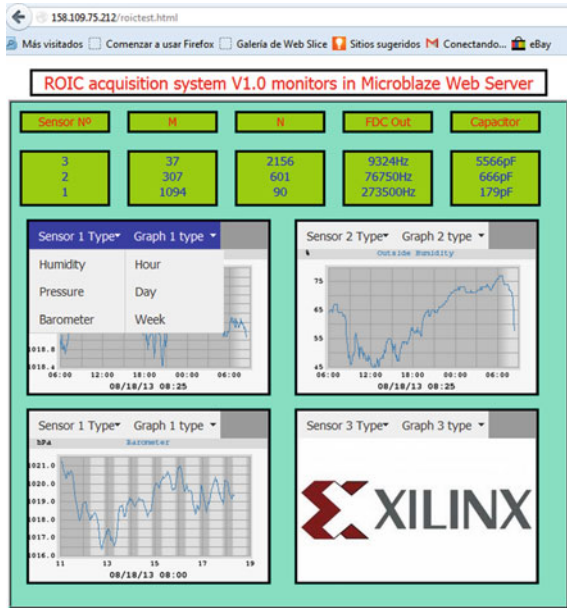
Fig. 10 Web site that allows to monitor the result of three different FDC channels and plot the results hourly, weekly or monthly
