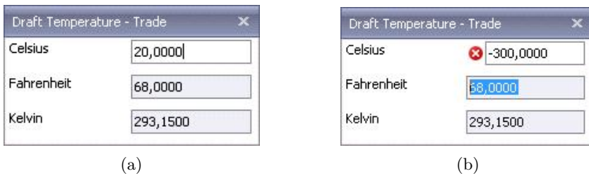
Fig. 3. Temperature typelet. Image (a) shows the typelet after evaluation of the update rule (upon change of the Celsius field). Image (b) shows the typelet after evaluation of the validate rule on invalid input (Celsius below -273.15 degrees).
