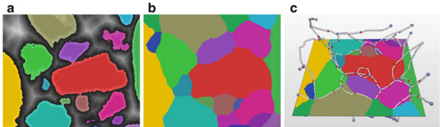
Fig. 3 Pore graph computation: (a) slice of labeled particles and distance information, (b) propagated particle regions, (c) pore graph constructed from the boundaries of the propagated regions. The colors of the graph elements correspond to Fig. 2
