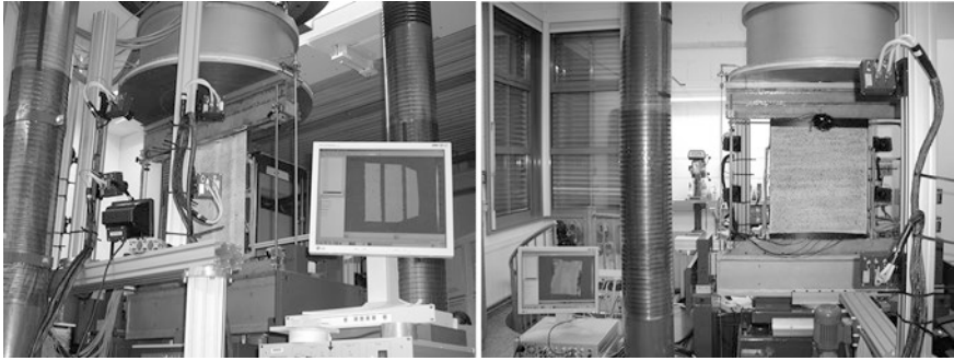
Fig. 11.5 Stationary ultrasonic equipment ( left ) and ultrasonic test setup for cylinders ( right )
