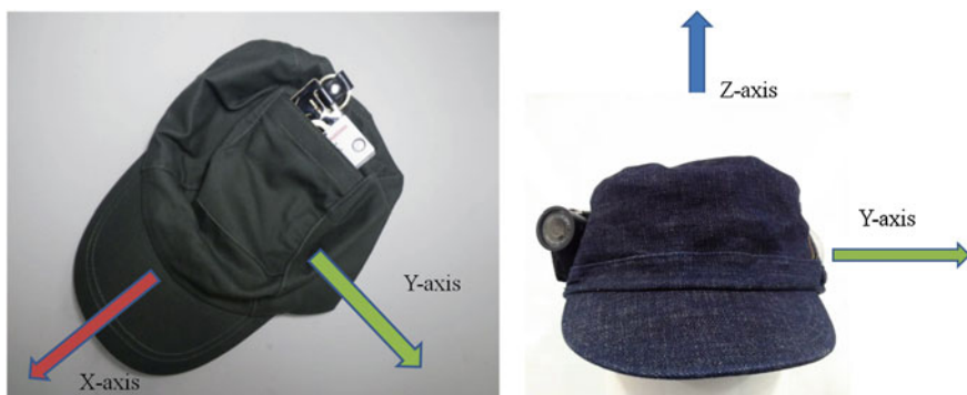
Fig. 5 A cap for mounting GPS and accelerometer loggers on the subject's head
