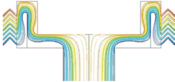
Fig. 1.16 Labyrinth as a noise silencer
