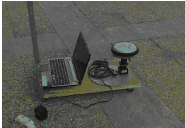
Fig. 23.6 Simultaneous positioning laser scanner and GPS on “mobile equipped trolley”
