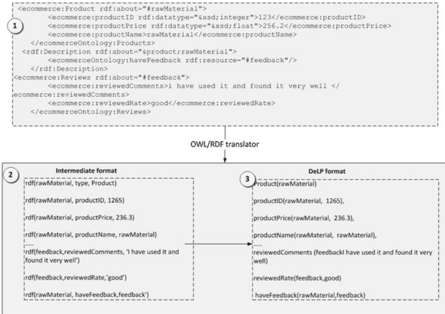
Fig. 5.9 Pictorial representation of the process for translation of information in OWL/RDF format to DeLP facts
