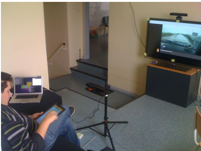
Fig. 2. Setup of the experiment with the user playing a puzzle game on the second screen (tablet) while a TV show is displayed on the main screen. The camera in the middle of the scene tracks head movements.
