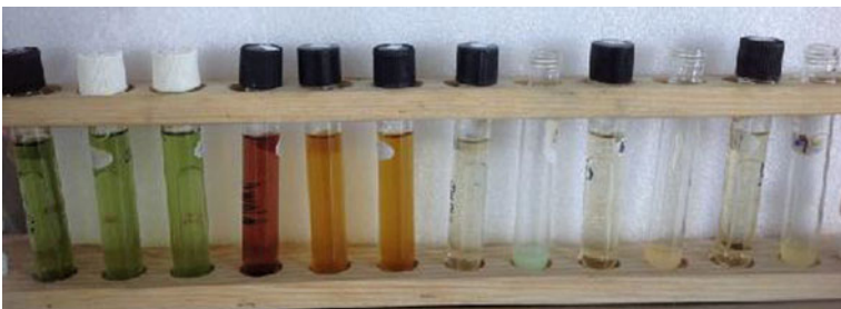
Fig. 3.6 Confirmative medium inoculated with the positive tubes from the presumptive tests
