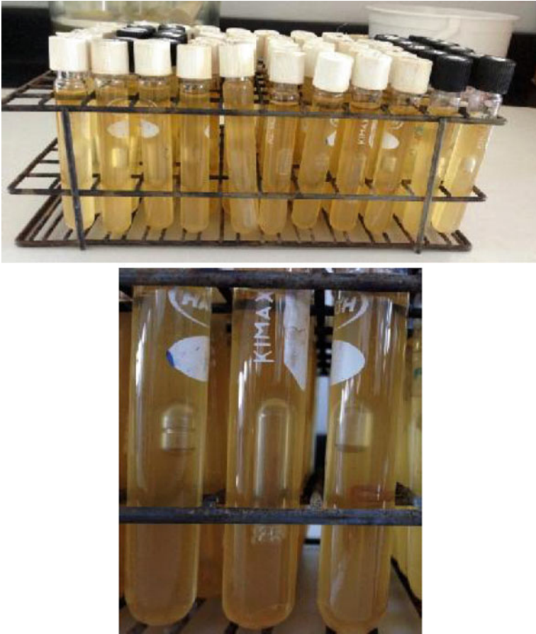
Fig. 3.5 Presumptive media inoculated with the disinfected water
