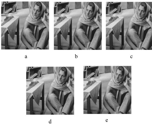
Fig. 5. (a) Original image, (b) Barbara image with SPIHT using CDF-9/7 for a bitrate of 3.0, (c) Barbara image with SPECK using CDF-9/7 for a bitrate of 3.0, (d) Barbara image with BISK using CDF-9/7 for a bitrate of 3.0, (e) Barbara image with TARP using CDF-9/7 for a bitrate of 3.0
