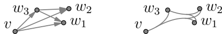
Fig. 5. Two drawings of the same graph. The absence of edge (w_1, w_2) is apparent because the curve from p_{w_1} to p_{w_2} is not smooth.
