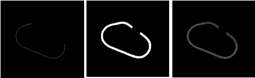
Fig. 10. Expected-state mask (left), current-state mask (middle), resulting match of both (right)
