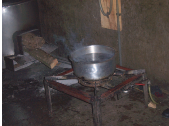
Fig. 15.3 Biogas cooking stove supplying a canteen close to Arusha (Diligent biogas plant). (Source: D. Rutz, WIP)
