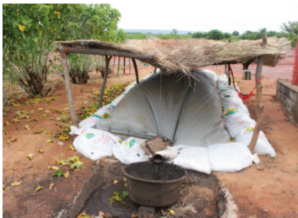
Fig. 11.3 Biogas plant at Mali Biocarburant SA (MBSA) in Mali. (Source: D. Rutz, WIP)
