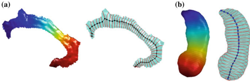
Fig. 4 Reeb graph computation via sampling level contours. a Left eigen-functions. Right Reeb graph as skeleton. b Left eigen-functions. Right Reeb graph as medial cores
