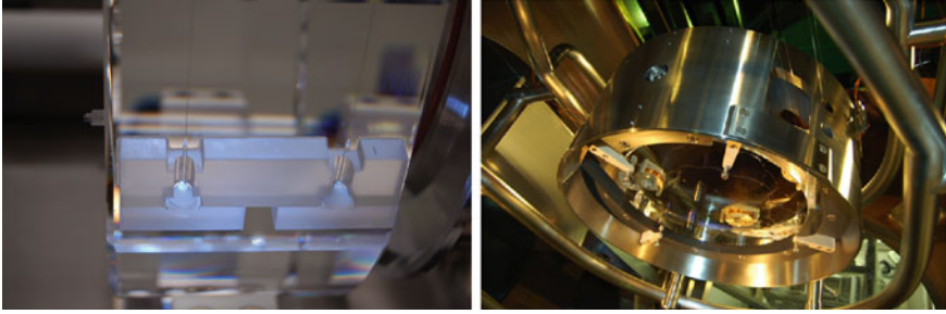
Fig. 1.8 The monolithic payload installed in Virgo in 2010
