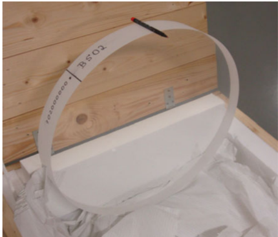
Fig. 1.7 The Advanced Virgo beam splitter
