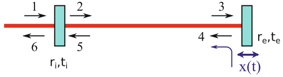
Fig. 3.6 Scheme of a resonant Fabry-Perot cavity with a moving end mirror
