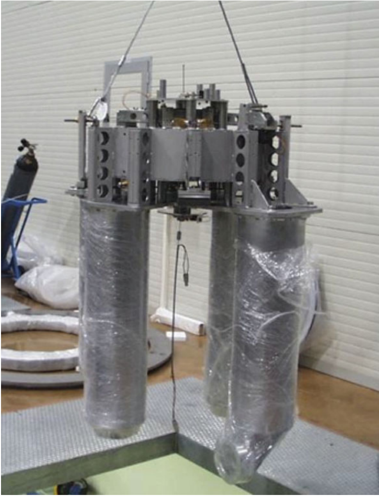
Fig. 7.9 The Filter 7 during the integration phase within a suspension chain of the Superattenuator. The four aluminum legs used as mechanical support for the actuation coils are visible. The first stepping motor used to rotate the system Filter 7-payload with respect to the upper part of the suspension chain is visible (platform for its installation) on top of the mechanical body. The second one, devoted to the payload rotation with respect to the Filter 7, is also visible on the bottom part filter body
